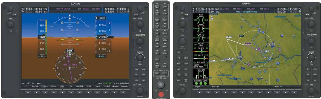
Figure 1-4 System Normal Operation
