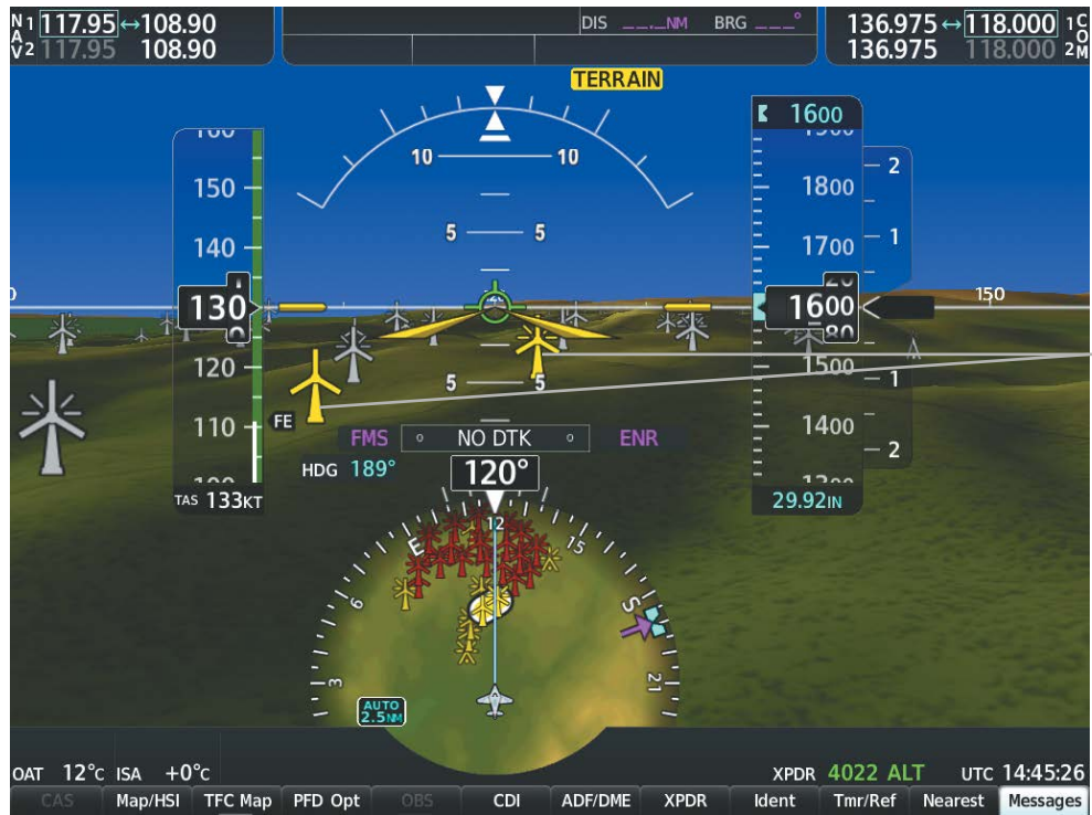
Figure 2-46 SVT with Obstacle Cautions
