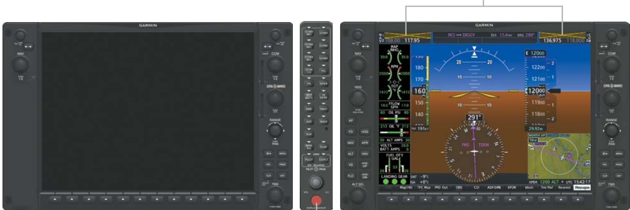
DISPLAY BACKUP Button Manually Activates/Deactivates Reversionary Mode on All Displays
