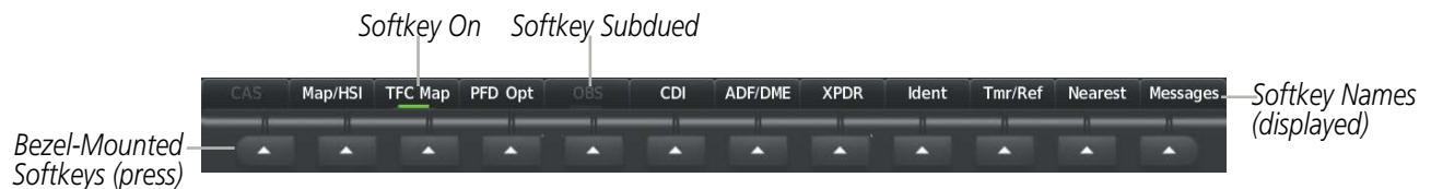
Figure 1-9 Softkeys (First-Level PFD Configuration)
