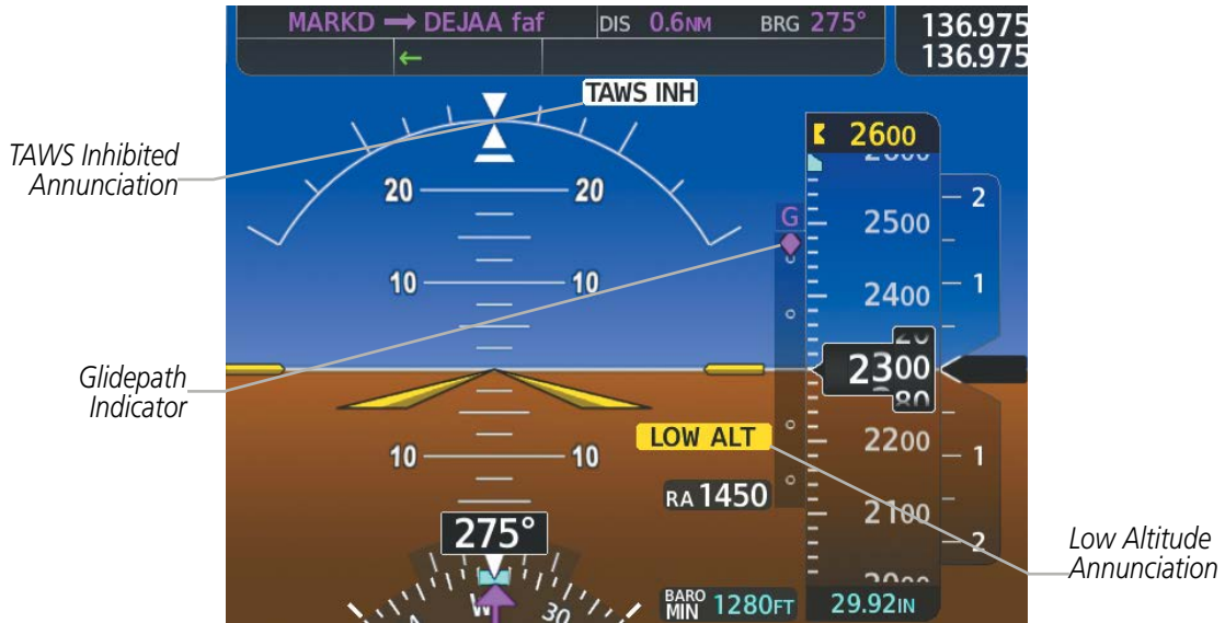
Figure 2-33 Low Altitude on GPS SBAS Approach
