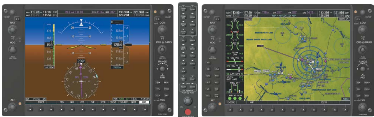
Figure 1-5 System Normal Operation
