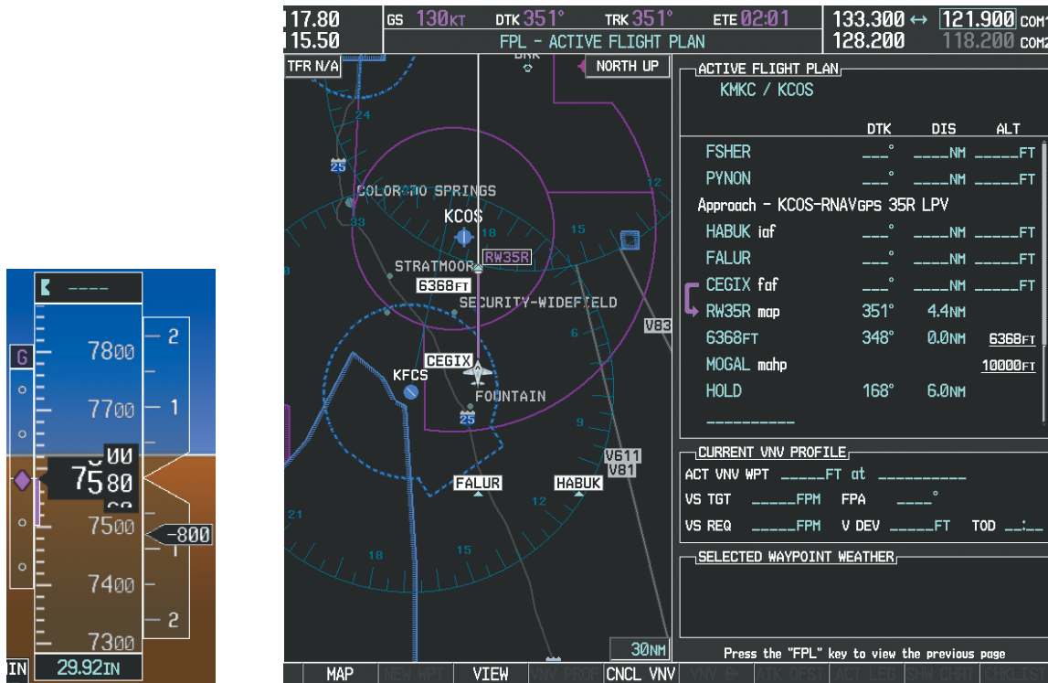
Figure 5-149 Descending to the Missed Approach Point
