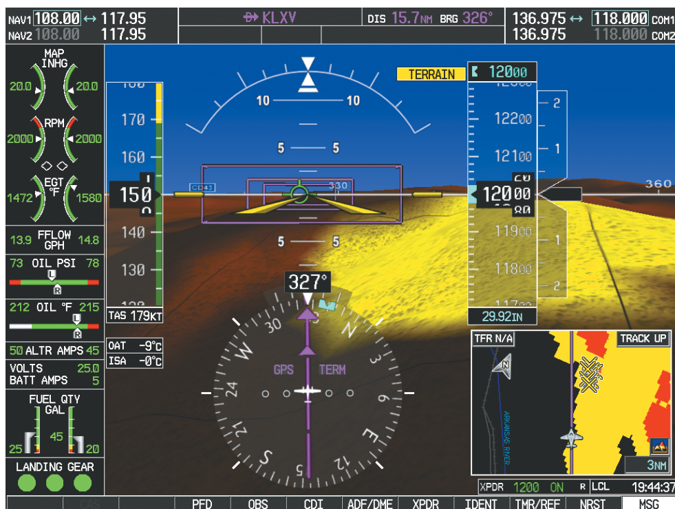
Figure 8-88 SVT Reversionary Mode
