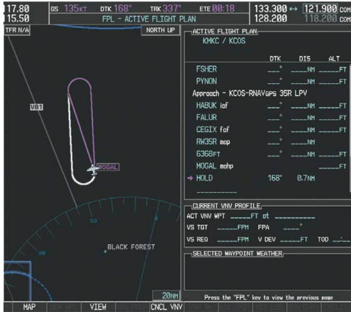
Figure 5-151 Establishing the Holding Pattern
