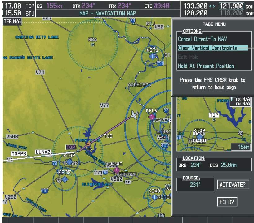
Figure 5-55 Direct-to Window - Clearing Vertical Constraints
