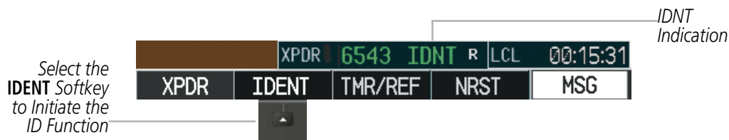
Figure 4-39 IDENT Softkey and Indication
